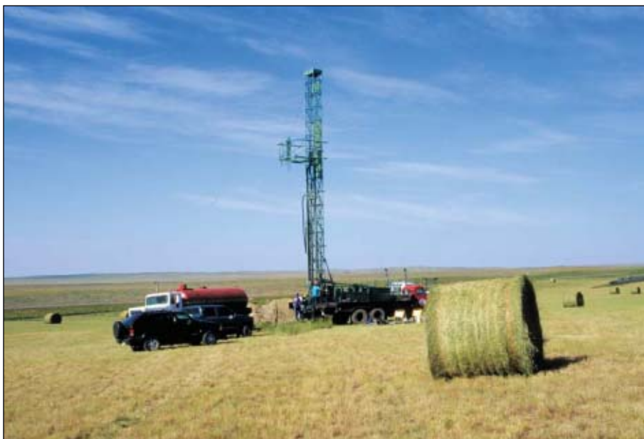
Truck-mounted rigs drills a coalbed methane well in the Powder River basin in Wyoming. Photo courtesy of Williams Cos.
